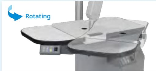
**The table rotates 90 degrees and the sliding bed for ARK is movable left and right**
